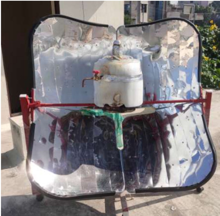
Fig. 2 Parabolic dish type solar cooker with heat storage unit
