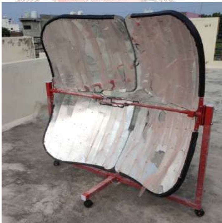
Fig. 1 Parabolic dish type solar cooker
